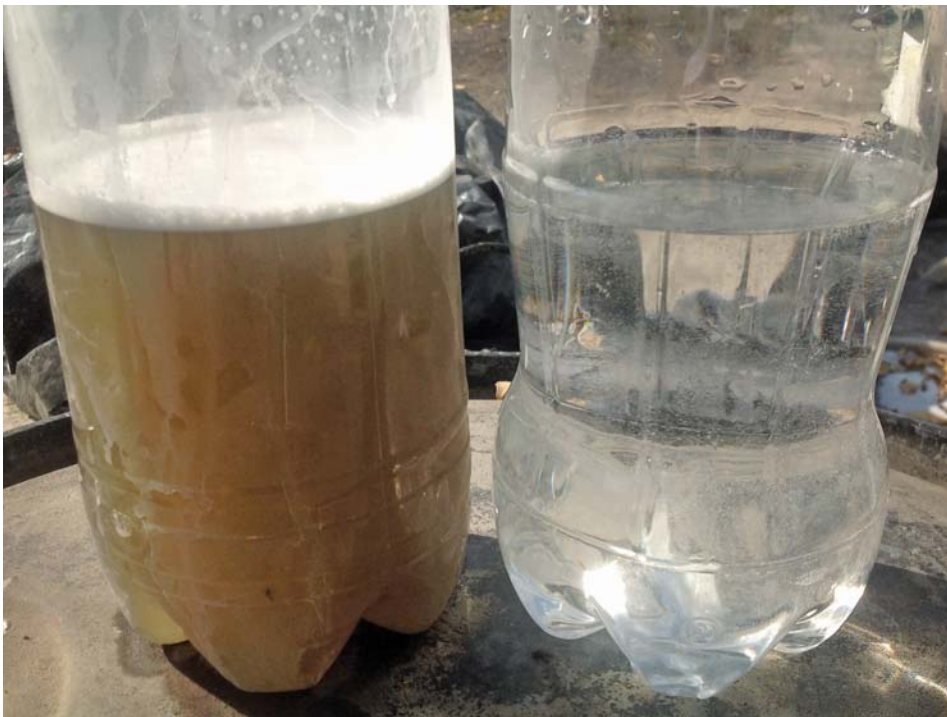
Feedwater and treated water from an oil processing company before and after undergoing its customized treatment process.
